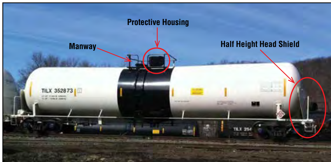
Example of a bare skinned or non-jacketed CPC-1232 tank car.
