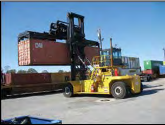
Intermodal container being lifted to put on rail car.
