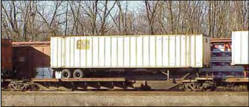
Flat car carrying trailer Also known as Trailer on Flat Car or TOFC
